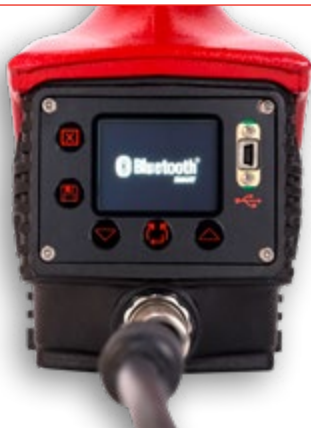
Built in Bluetooth® for wireless data transfer
