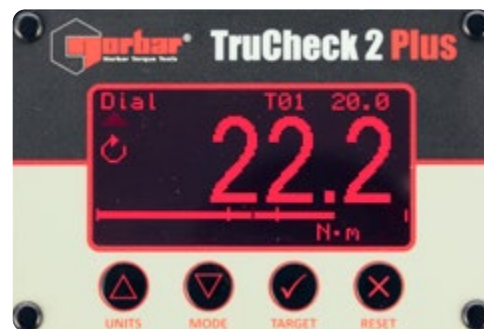
TruCheck™ 2 Plus display showing above target tolerance
