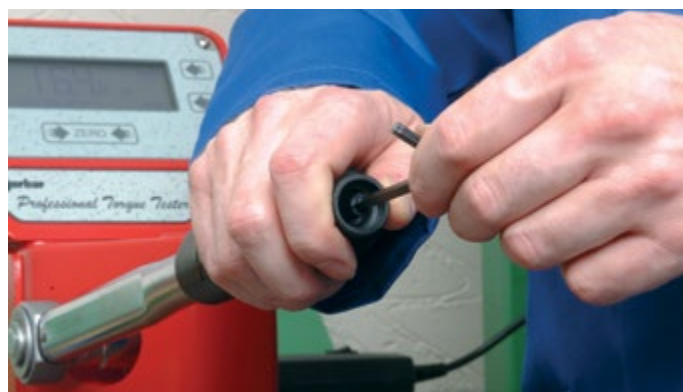
Setting a 'P' Type Torque Wrench
