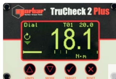
TruCheck™ 2 Plus display showing below target tolerance
