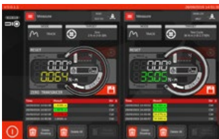
Displaying 2 transducer readings simultaneously
